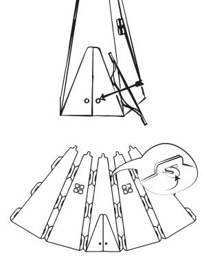
Place the body parts next to each other, in the order shown. Fasten the pieces together using the connectors as shown.
