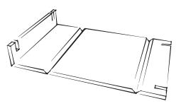
**3.** Take part B and fold up the end that is attached to the short center face. (2x)
