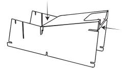
3. Slide housing B into the sides through the slots.
