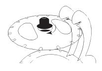
Twist the socket of the lamp into the hole of part D.
