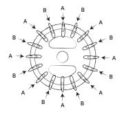
Slide parts A and B alternately into the slots of parts C and D.
