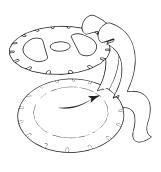
Slide part C into the remaining slots of part A and part B.
