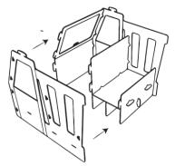
Attach side A to partition wall I, back H and front B.
