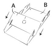
4. Slide part A into the first slot of B.
