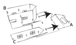
Slide the side walls B and C of the housing into the appropriate cutouts in part A.
