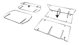
Fold the shelves and the side walls over the fold lines as shown (4x)
