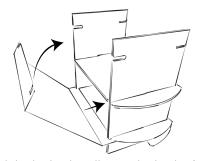
Slide the back wall onto the back of the bottom shelf. Then attach the top.
