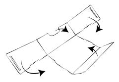
Prepare the drawer by folding it over and inserting the bulges into the slots. Slide it into the bottom box.
