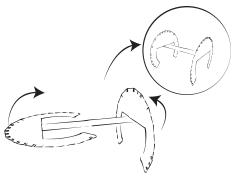
Take both parts A and fold the curved parts on the folding lines 90 degrees.
