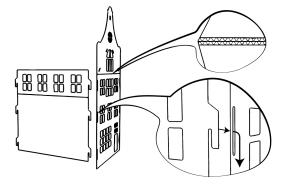
Make sure the cuts are on the outside of the house and then hook the sidewalls into the cutouts in the front wall.
