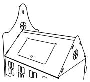
Clamp the roof between the front and back walls by clicking the protrusions of the roof into the cutouts.
