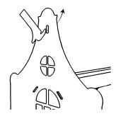
Hook hoist part 1 into the slot in the front wall.
