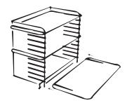
Slide parts B into the upper, middle and lower incisions of A.
