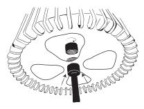
Remove the ring from the lamp base, then insert the lamp base D into the middle circle of part B and tighten the ring.
