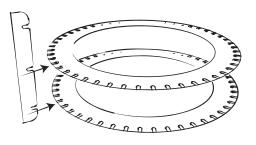
Insert a part C into the incisions of the middle part A and down part A
