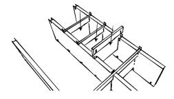
Fold the narrow planks E over the fold lines and slide them into the other cuts in the walls.
