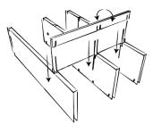
Fold the wide plank D over the fold lines and slide it into the incisions at the bottom of the vertical walls.
