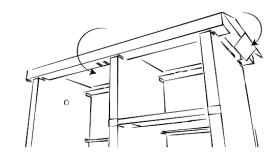
Attach top G to the cabinet by folding the flaps over. Do the long sides first and then the short sides.
