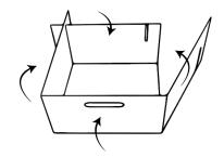
Fold the tray in over the fold line and slide the sides into the slots in the back.
