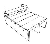
Fold the back parts F over the fold lines and slide into the cuts in the back.
