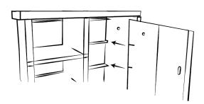
Slide the doors between the outer walls as shown. Then follow step 11 and proceed to step 13.
