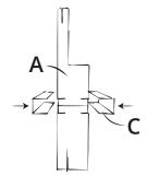
Slide parts C into both sides of parts A to hold the structure together.
