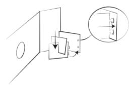
2. Slide parts I and J together and slide them in part A. Then slide parts into I and K and slide them into place in part B.
