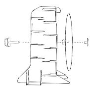
Add the rotating plate D by attaching it through the cap in the hole of the middle cross-beam.
