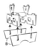
Now slide the support beams B into the frame.
