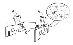
Place the frames A opposite each other and slide support beam C between them. Secure it with locking piece F.
