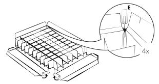
Fold the flaps at the corners, fold up the sides of the bed and attach them with the corner clamps E.
